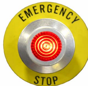
E-Stop activated. (LED illuminated)
