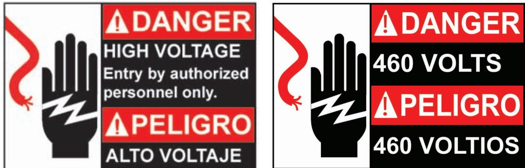
Figure 2-1 - Red & Black labels indicate DANGER hazards
